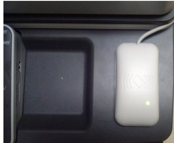
4. Registering your ID card is the preferred method of accessing machine functions. To start, simply hold your card one half-inch or less from the reader. The reader will beep, indicating the card has been read.
