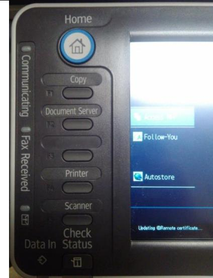
13. If a hard function key is pressed before logging in, this screen is displayed. A registered card can be swiped from this screen and after a few moments the function screen will become active.
